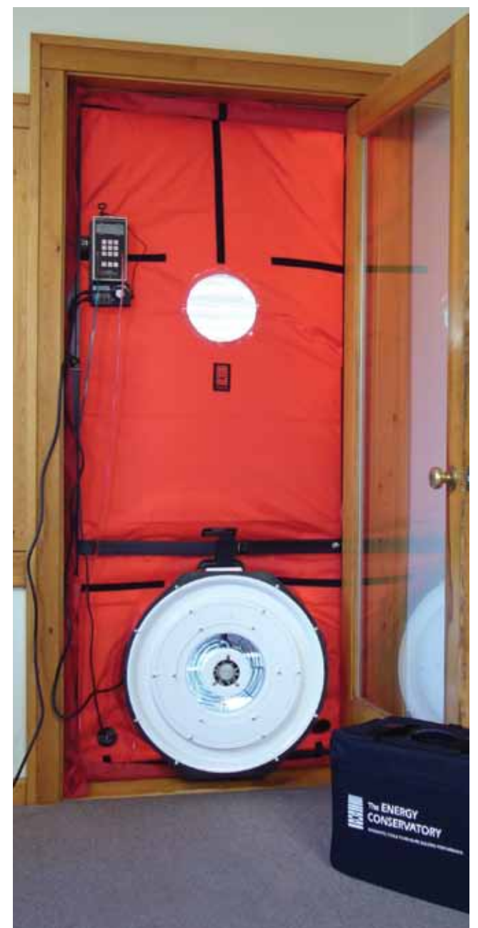
Fig.3: Minneapolis blower door test
